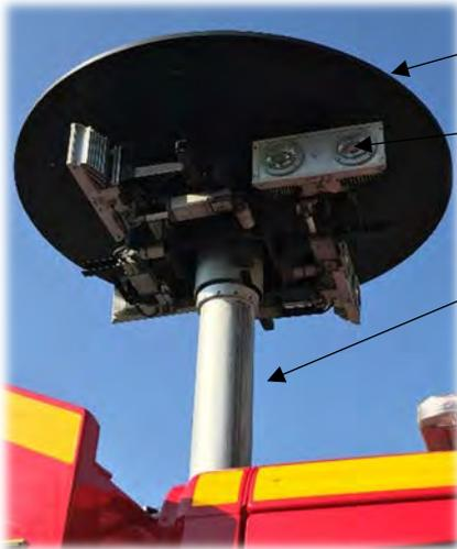
PLATEAU TÉFLON ISOLANT
