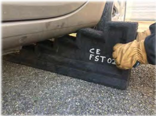
ENGAGER LA CALE SOUS LE VÉHICULE JUSQU'À L'AMENER EN CONTACT
