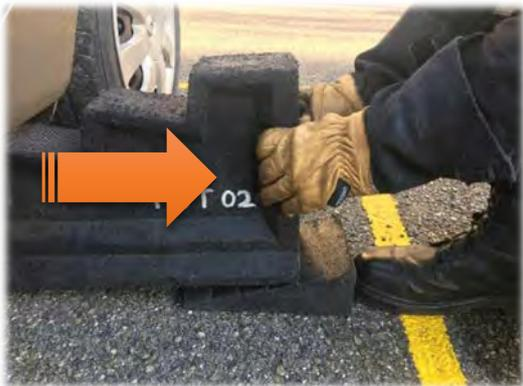
METTRE SON PIED EN OPPOSITION DU COIN À MARIER POUR NE PAS QU'IL GLISSE, PUIS EXERCER UNE LÉGÈRE TRACTION SUR LA CALE POUR L'AMENER EN CONTACT AVEC LE VÉHICULE ET INHIBER LA SUSPENSION.
